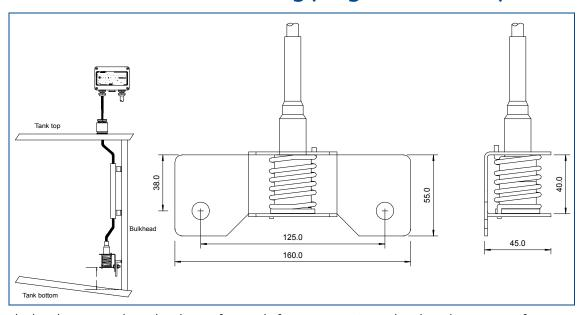
The brackets are U-shaped and manufactured of 2 mm ASTM 316L plated steel. Diameter of mounting holes: 11.5 mm. The transducer is secured by means of a spring fitted into two holes in the "U" shape, and can be mounted/dismounted without the use of tools.
